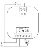
Install the product in the appliance box behind the push button/box lid or secure it with a Mounting clip (MNT-01, not included) on the wall or DIN rail.
