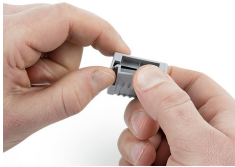
Open the Gelbox at the side latches.
