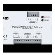
With the PROLED AMPLIFIER (12-24 V) you can boost the PWM signal with additional 4x 8 A. For the AMPLIFIER you need an additional switching power supply (12-24 V). 3 versions are available (CA to CA, CC to CC und CA to CC). By using the version "CA to CC" the PWM input signal is common anode
