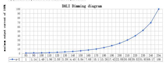
target dimming stage of the total 254 stages
