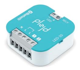
LED Driver 10 W with built-in dimming function for one or more LED luminaires (150–700 mA) or LED strips (12/24 V DC) for up to 10 W. The product can be controlled wirelessly via the app or through other products from Plejd.
