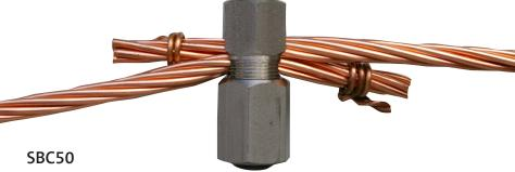
Elpress's simple and safe stainless steel screw branch clamp SBC50 makes it possible to branch off a reinforcement bar with a stranded earth wire in copper or steel. The screw branch clamp can be used to satisfy many different types of earthing needs, such as earth electrodes, ring earthing, foundation earthing, equipotential bonding, lightning rods. The clamp provides good direct contact between the conductors.
