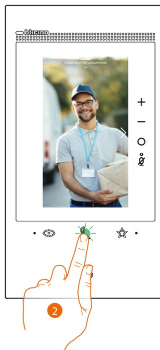
2. The communication LED flashes, touch the communication key to activate the audio communication.
