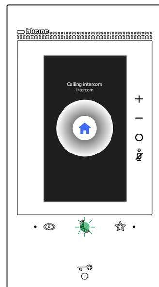
2. Touch to activate the intercom with the desired Internal Unit.
