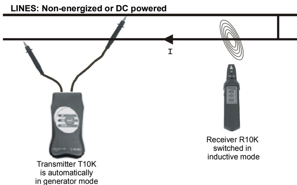
**Fig. 7. Injection of test current into tested loop**
