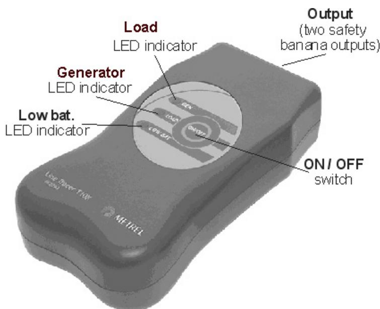
**Fig. 1. Transmitter T10K**
