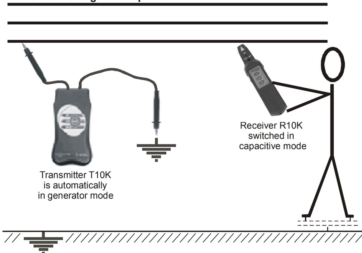
**Fig. 9.** Tracing the electrical field of a line
