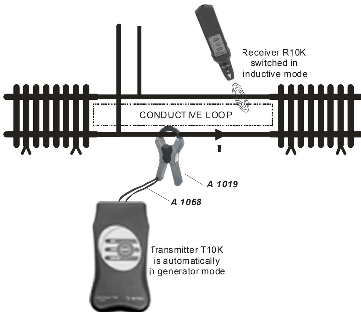
**Fig. 18.** *Tracing conductive loops by using current clamp*
