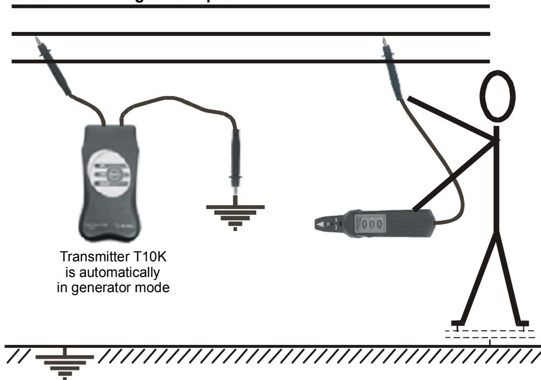
**Fig. 10.** Tracing the conductor using Test tip
