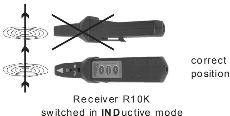
**Fig. 4.** Detection of electromagnetic field
