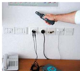
With various arrangements a detection depth between 40 and up to 200 cm can be reached on energized lines, a detection depth up to 40 cm can be reached on non-energized lines.
