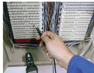
This locating method requires the use of a test tip which is part of a standard set. The high accuracy of the method allows for pinpoint determination of a traced conductor.
