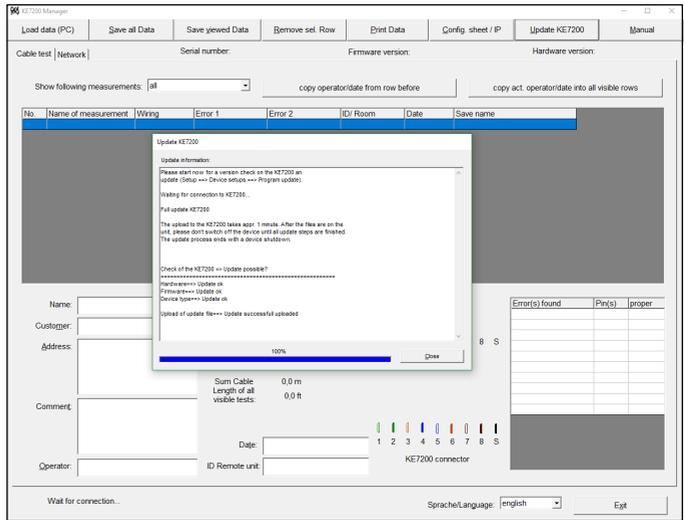
**Configurations: The KE7200/KE7100 is supplied with 15 predefined wiring definitions and 16 predefined cable variants. New definitions can be created or existing ones revised at any time in the setup.**
