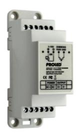
1 channel LED dimmer. Control is either via a 100 k $\Omega\square$  potentiometer, 1–10 V control voltage source or with a push button (PUSH-DIM function). The output voltage corresponds to the supply voltage of 12–24 V.
