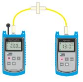
Now disconnect the measuring cable from the power meter and connect the open end via a coupling, e.g. to the fibre section to be measured. The other end of the fibre path is now connected to the level meter. Make sure that the connection at the power level transmitter is not detached or altered.
