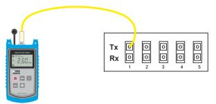
Connect the KE8000 level meter directly or via an optical measuring cable to your test object.
