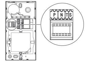
For the Classe 100 and Classe 300 internal units, the S configurator associates the entrance panel to the bell programmed in the internal unit.
