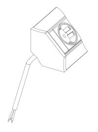
End cap with power input and/or output connector.
