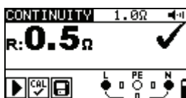
Figure 5.12: Example of a continuity test
