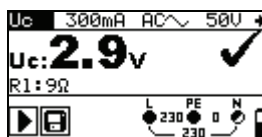
Figure 5.18: Example of a contact voltage measurement
