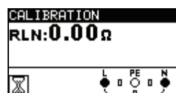
Figure 5.15: Result after calibration
