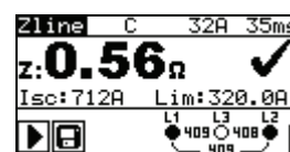
Figure 5.29: Example of a line impedance measurement
