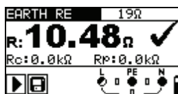
Figure 5.35: Example of an earthing resistance measurement
