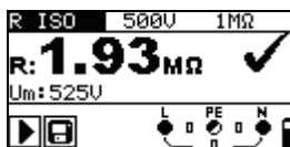
Figure 5.7: Example of an insulating resistance measurement
