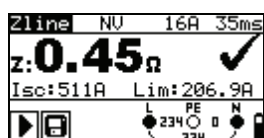
Figure 5.29: Example of a line impedance measurement
