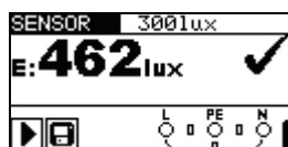
Figure 5.47: Example of a luminous intensity measurement
