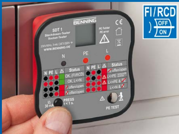
Testing the tripping function of a 30 mA RCD by pressing the FI/RCD TEST key
