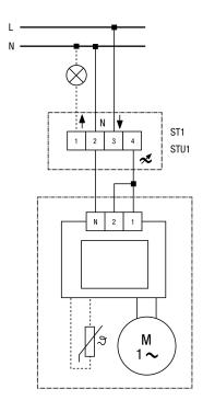
ST 1 - Speed controller (AP) STU 1 - Speed controller (UP)
